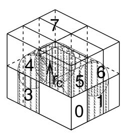
Fig. 5.11: A non-staggered domain decomposition grid of  $3\times2\times2$  cells. Coordinates in zones 1 to 7 are communicated to the corner cell that has its home particles in zone 0.  $r_c$  is the cut-off radius.
